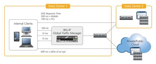
Figure 5: BIG-IP GTM enhances user experience through scalable, high-performance DNS caching and resolving.
