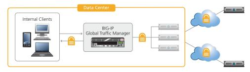
Figure 7: BIG-IP GTM is the DNS resolver responsible for requesting the additional DNSSEC records and doing the crypto calculations to validate that the DNS response is correctly signed.
