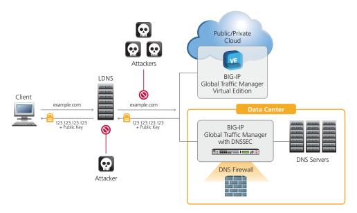
Figure 6: BIG-IP GTM with DNSSEC delivers real-time signed DNS query responses to clients.
