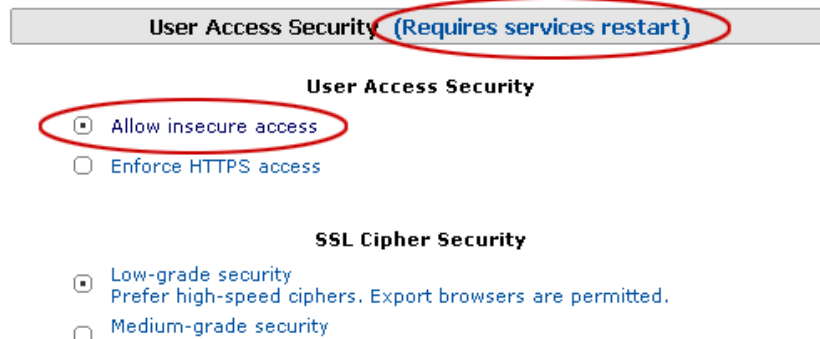
Figure 4 Allowing insecure access so the BIG-IP LTM can offload the SSL traffic
