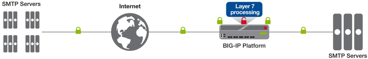
4. **SMTP encrypted with TLS/SSL on both client and server sides**
