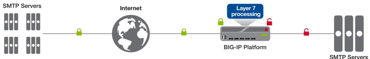
Figure 2: SMTP encrypted on the client-side only
