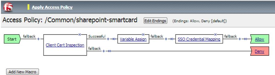
Figure 7: Client Certificate VPE example
