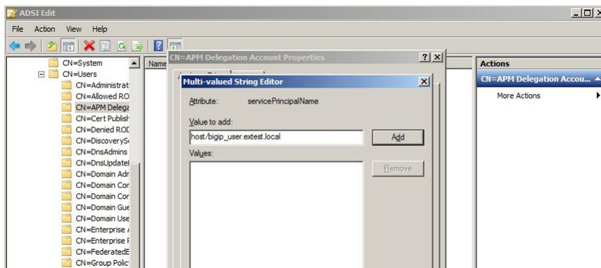
Figure 4: Adding the user to the servicePrincipalName
