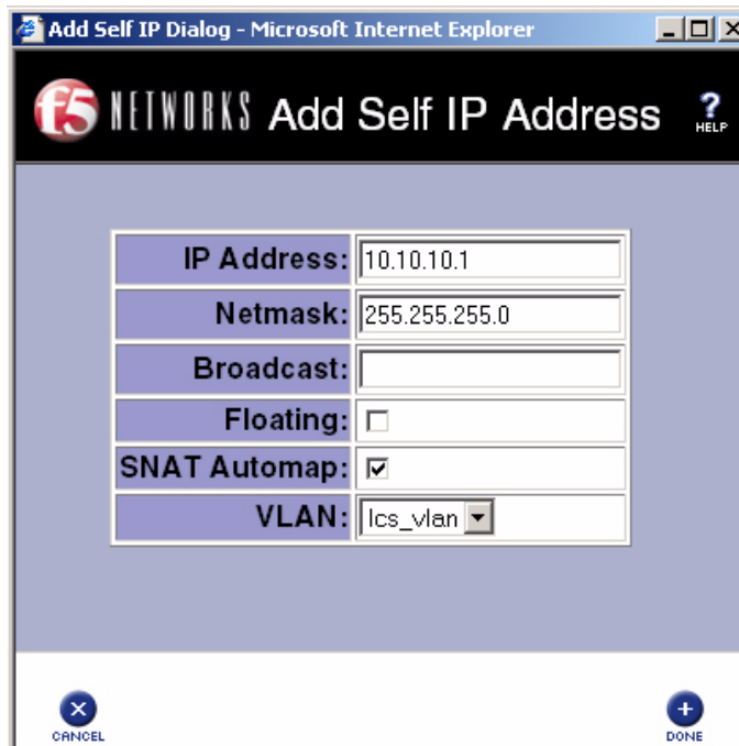
Figure 1.3 Adding a self IP address in the BIG-IP Configuration utility
