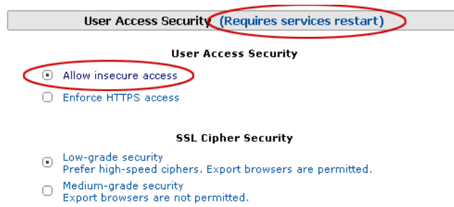
Figure 4 Allowing insecure access so the BIG-IP LTM can offload the SSL traffic
