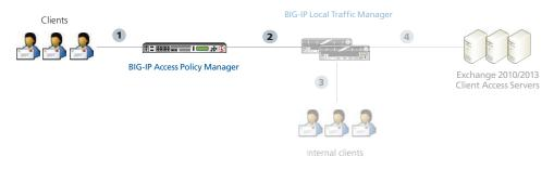
1. HTTP-based Client Access traffic goes to the BIG-IP APM, which provides proxy authentication and secure remote access.
