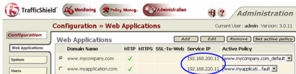
Figure 1.2 The finding the Web Application Service IP in the TrafficShield user interface.
