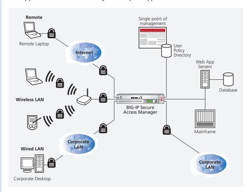
Creating multiple virtual BIG-IP Secure Access Manager instances (virtual IPs) enables the consolidation of different unified access groups onto one device.
