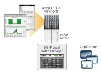
F5 products deliver a probe-less deployment of high speed logging of syslog data to PresiNET TOTAL VIEW ONE, which is used to create enhanced network and application visibility reports.
