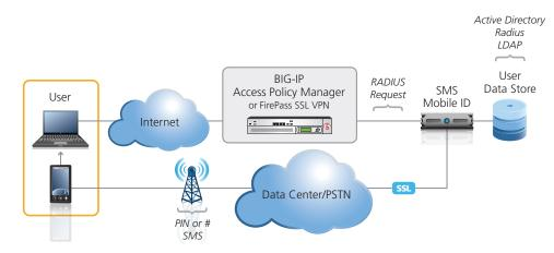
SMS Passcode provides strong authentication with one-time passwords over mobile phones for user authentication with BIG-IP Access Policy Manager and the FirePass SSL VPN solution.
