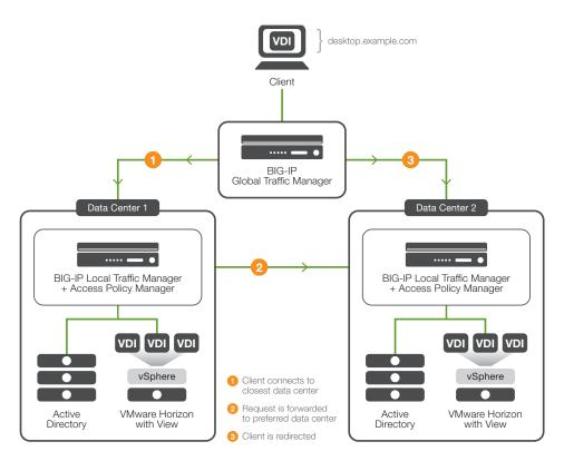
Example of a simplified single namespace architecture for VMware Horizon with View.
