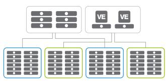
Figure 5: ScaleN scales across applications, not servers, and enables elasticity of BIG-IP services across virtual and physical instances in a Device Service Cluster.
