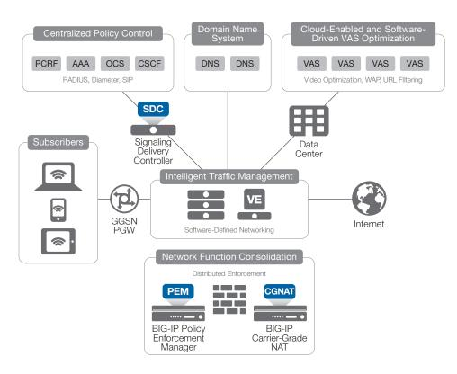
Figure 3: VAS bursting in a virtualized CSP network with F5 products
