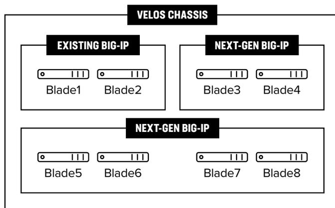
**Figure 1:** VELOS enables customers to host different BIG-IP software tenants on the same chassis.
