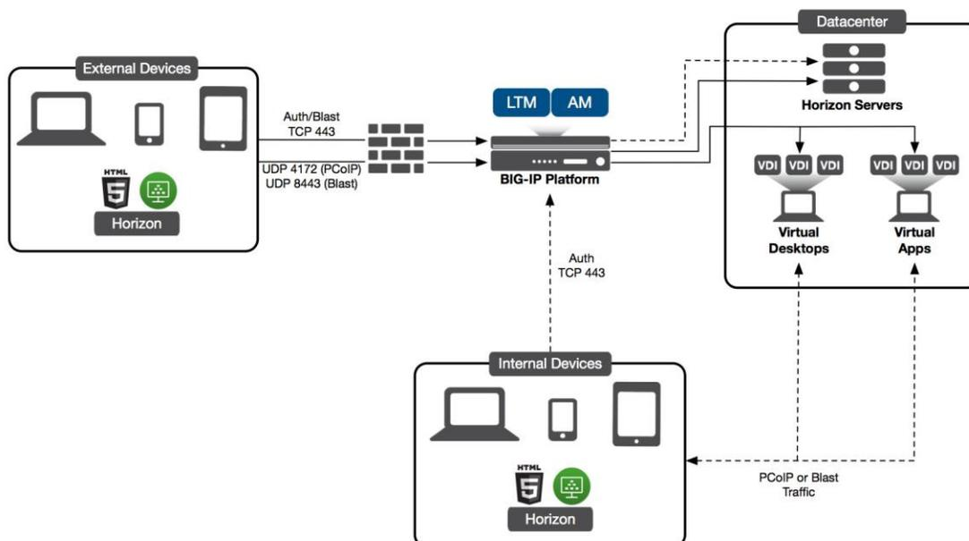
For deployments with the BIG-IP system fully proxying PCoIP/Blast traffic and Connection Servers, the traffic flow is (grey callouts)
