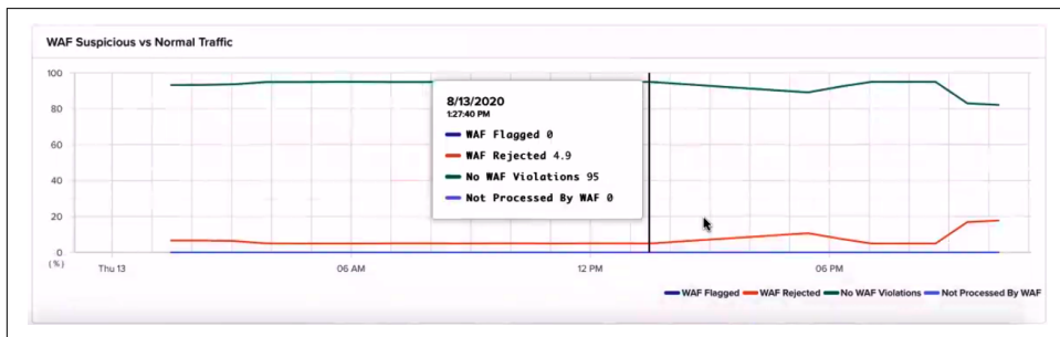
Figure 7-2. Controller ADC comparing normal traffic versus suspicious or blocked traffic.
