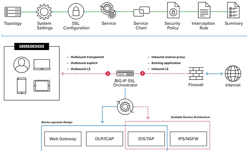
The powerful classification engine of BIG-IP SSL Orchestrator applies different service chains based on context derived from:
