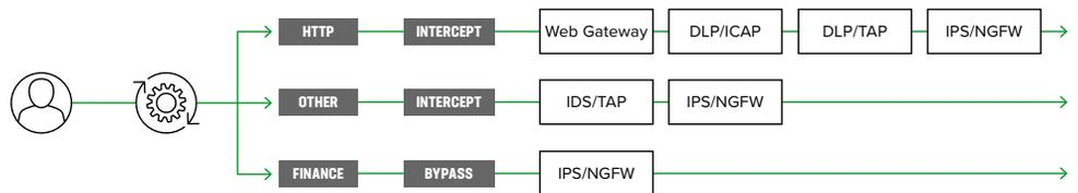
Each service chain is linked to service chain classifier rules and processes specific connections based on those rules, which look at protocol, source, and destination addresses. Service chains can include each of the three types of services (inline, ICAP, or receive-only), as well as decryption zones between separate ingress and egress devices.
