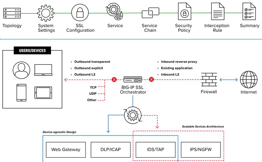
BIG-IP SSL Orchestrator enables administrators to apply different service chains based on context derived from a powerful classification engine. That context can come from:
