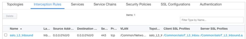
This completes the configuration of BIG-IP SSL Orchestrator as a forward proxy. At this point an internal client should be able to browse out to external (Internet) resources, and decrypted traffic will flow across the security services.
