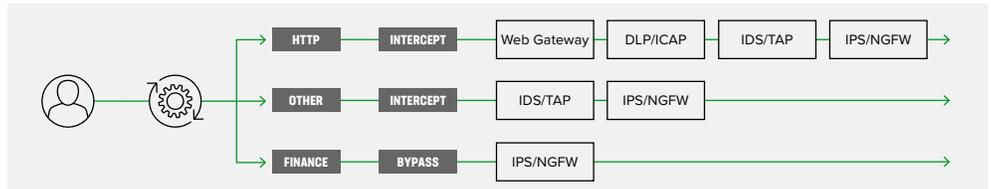
Each service chain is linked to service chain classifier rules and processes specific connections based on those rules, which look at protocol, source, and destination addresses. Service chains can include each of the three types of services (inline, ICAP, or receive-only), as well as decryption zones between separate ingress and egress devices.
