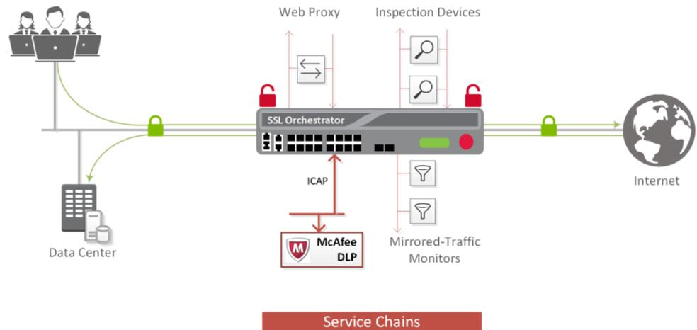
Figure 6: The McAfee DLP system in a BIG-IP SSL Orchestrator service chain architecture.
