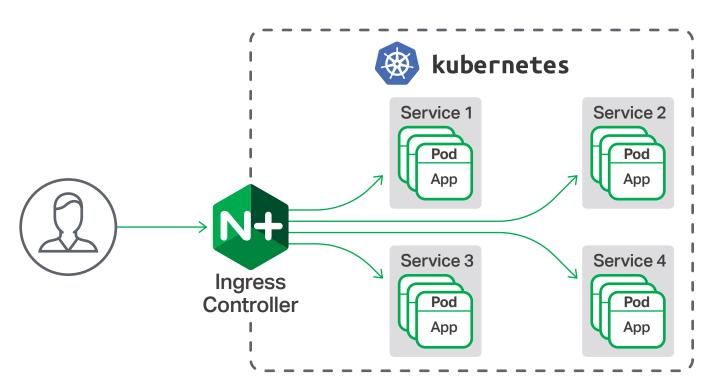
Use the NGINX Ingress Controller for Kubernetes for SSL termination, routing, and load balancing
