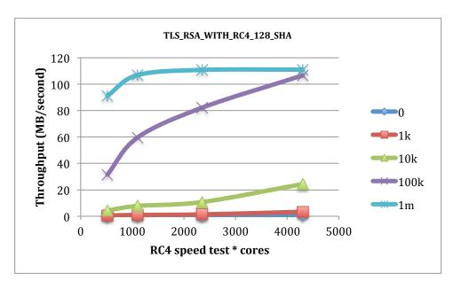
Note that even the low-powered machines in the test quickly saturated the 1 GbE network when using the RC4 bulk cipher.
