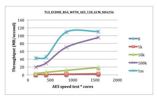
Determining a correlation between bandwidth and AES speed is more challenging because the test network was only 1GbE-capable (approx. 111MB/s effective throughput), and because bulk ciphers such as AES are relatively efficient; the performance of the cipher does not have a significant bearing on the performance of the system.
