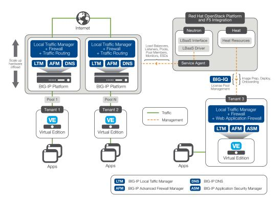
Figure 1: F5 OpenStack deployment test architecture
