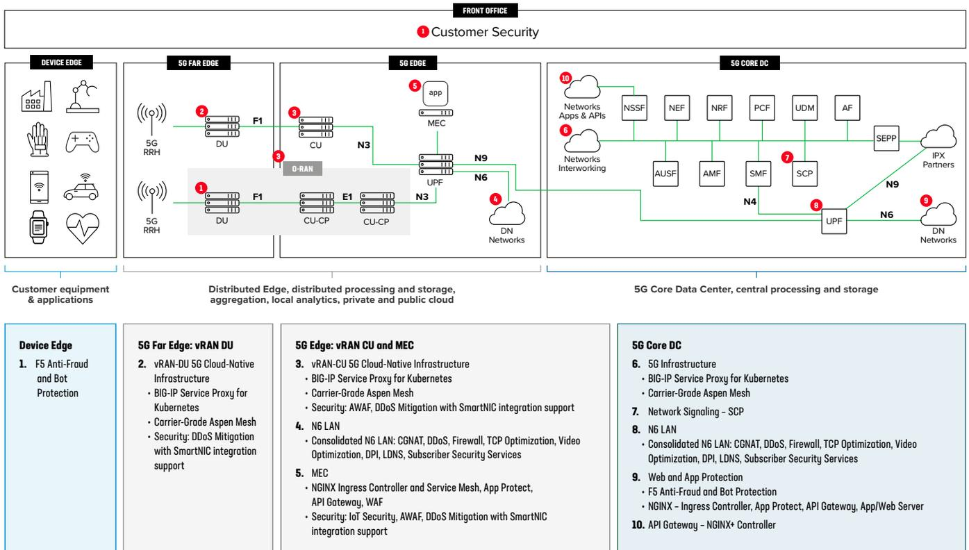
Figure 2: F5 security solutions for service providers
