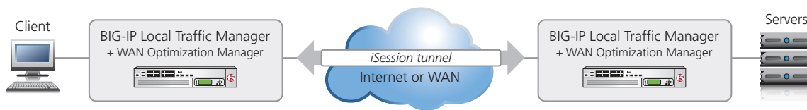
Figure 3: Symmetric BIG-IP WOM devices optimize and secure traffic over the Internet.
