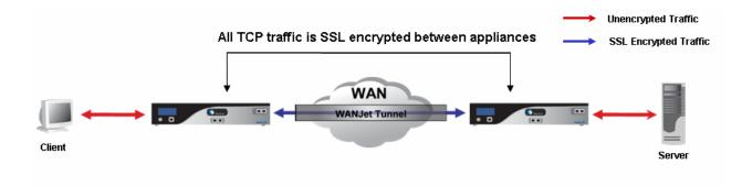
You can deploy WANJets at either end of the SSL tunnel to maintain security for insecure traffic over the Internet. WANJet also gives you the option of selectively encrypting certain types of traffic.
