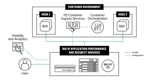
**Figure 1:** F5 Container Ingress Services deploys in container environments, enables self-service selection in orchestration, and subscribes to events to create, scale, and remove app services. You can also export your data streams for more in-depth visibility, observability, and analytics.
