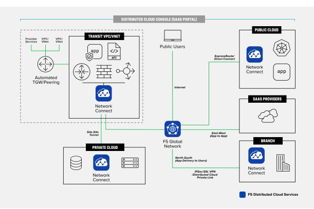
**Figure 3:** A visual look at how multi-cloud transit works inside Distributed Cloud Network Connect
