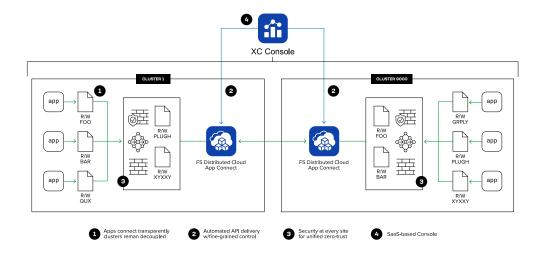
**Figure 2:** An architectural view of F5 Distributed Cloud App Connect, which reduces the time and complexity in connecting applications across public and private clouds.
