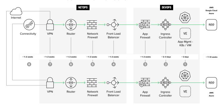
**Figure 1:** A graphical depiction of the steps involved in delivering an application across multiple clouds using conventional tools and cloud providers.
