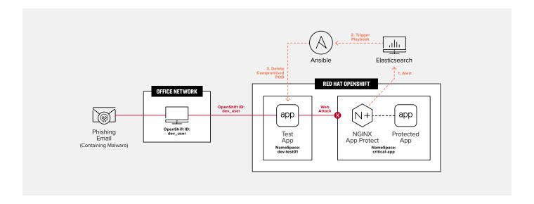
Figure 2: NGNIX App Protect, Elasticsearch, and Ansible can be tightly integrated to deliver powerful, automated threat remediation.
