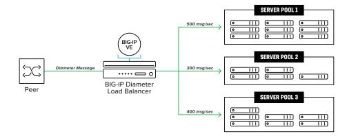
Figure 1: Diameter traffic management—load balancing.
