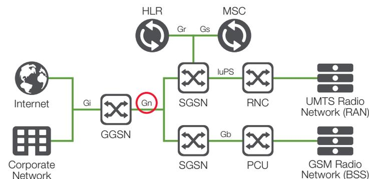
Figure 1: An example of a 3G network; Gn (circled in red) is a GTP-based interface.
