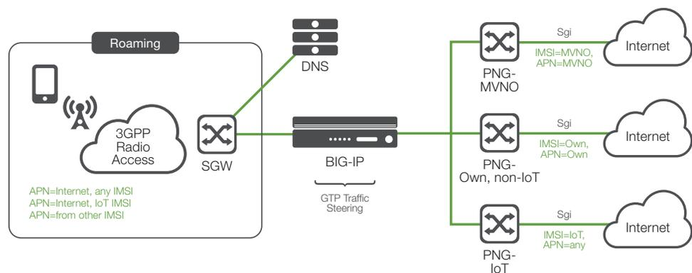
**Figure 2:** GTP Proxy—Correct APN and route on IMSI range.
