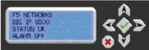
The LCD panel is located on the front of all F5 hardware except for the Viprion 2400 Series Chassis. A separate USB attachable LCD panel is available for the Viprion 2400 Series Chassis.
