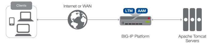
Figure 1: Using the BIG-IP system as a reverse proxy
