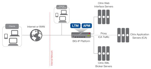
Figure 4: Using the BIG-IP APM with Web Interface servers
