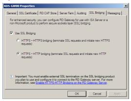
Figure 2: Configuring HTTPS-HTTP bridging on the TS Gateway server
