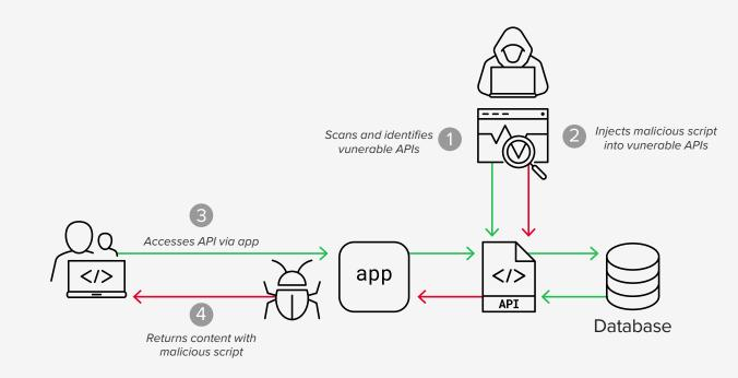
**Figure 3:** APIs can be embedded deep within business logic yet remain susceptible to attack.
