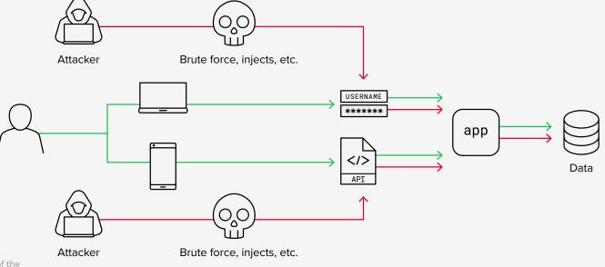
Figure 2: APIs are susceptible to many of the same security vulnerabilities as web applications.
