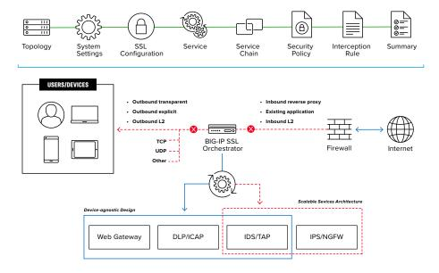
BIG-IP SSL Orchestrator enables administrators to apply different service chains based on context derived from a powerful classification engine. That context can come from:
