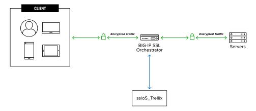
This completes configuration of BIG-IP SSL Orchestrator as a forward proxy. At this point an internal client should be able to browse to external (Internet) resources, and decrypted traffic will flow across the security services.
