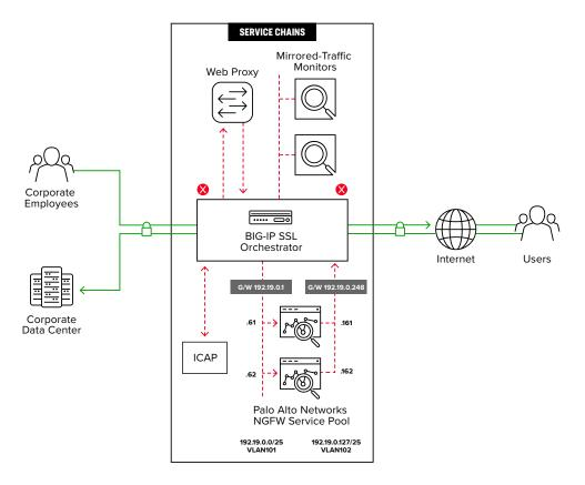
**Figure 10:** An L3 service deployment architecture
