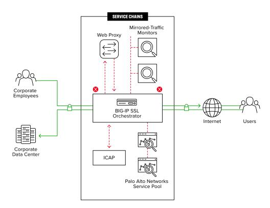
Figure 4: A sample inline deployment architecture
