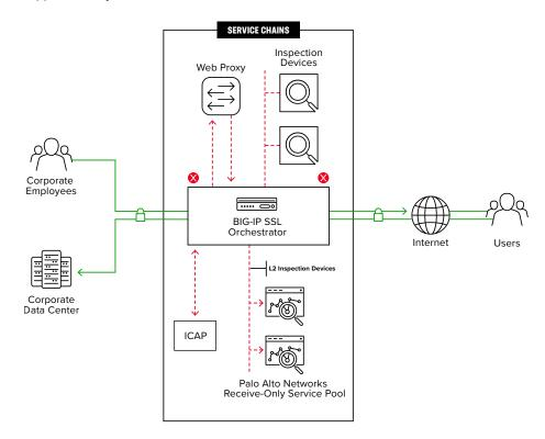
**Figure 11:** A TAP service deployment architecture
