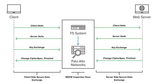
**Figure 1:** The F5 full proxy architecture
