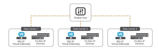
Figure 1: BIG-IP devices across various data centers can be configured and managed by an Ansible host.
