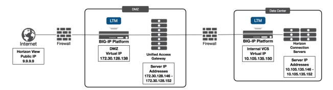
As part of the workflow, the configuration has LTM placed in the front and behind the Unified Access Gateway (UAG) Servers. This is because in production scenarios, multiple UAG servers require load balancing. Connection servers that manage the Horizon environment in the datacenter must also be load balanced to prevent Single Points of Failure (SPoF).
