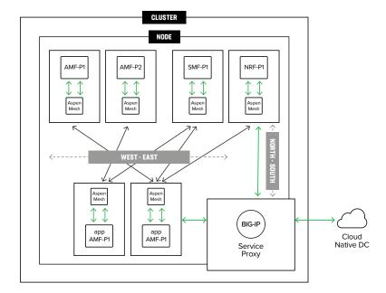
**Figure 1:** F5 Service Proxy for Kubernetes and Carrier-Grade Aspen Mesh deployment option.
