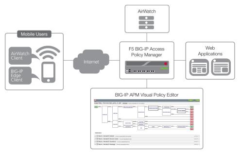
Integrating AirWatch with BIG-IP APM enables organizations to customize user access policies based on mobile device configuration.
