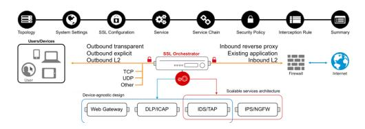
Figure 2: BIG-IP SSL Orchestrator enables dynamic service chaining based on user-defined policies..
