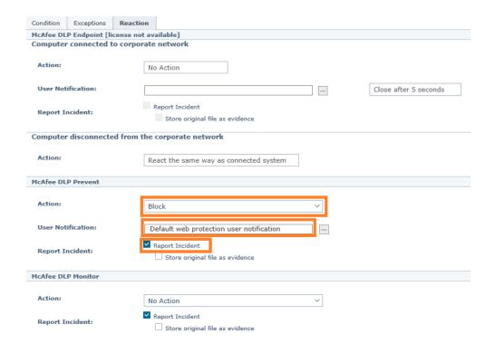
Figure 4: Example configuration for reaction to a policy rule violation, in the McAfee ePO system.
