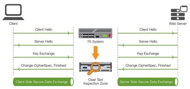
Figure 1: The F5 full proxy architecture
