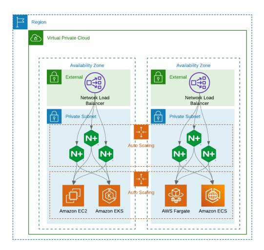
As an alternative, NGINX Plus can be deployed in an external subnet with Public IPs assigned to each instance in the Auto Scaling group. In this kind of deployment, GSLB can be used to disaggregate the client traffic to the instances without the need for ELB. Note: GLSB should be configured to subscribe to the list of public IP addresses associated with each instance in the Auto Scaling group, emit low-TTL responses, and use health checks to validate the health of each instance.
