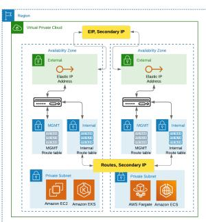
When applications are deployed on EC2 instances it is like when they are deployed into a data center. The EC2 instances become pool members on BIG-IP instances running in AWS, your data center or at a Cloud Interconnect location. For more details, please see the F5 GitHub.
